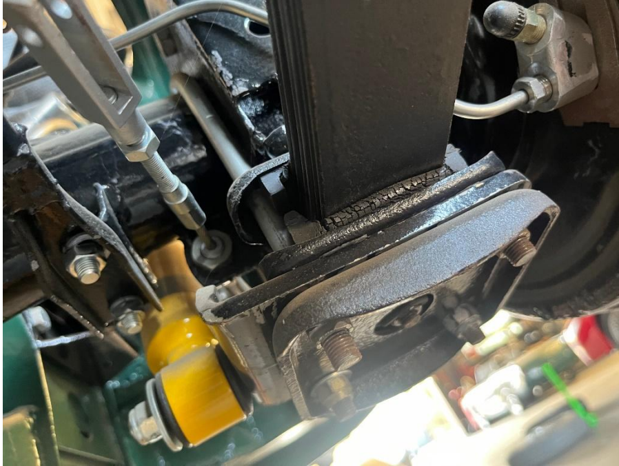
Installation showing original lower plate reused (preferred method)
