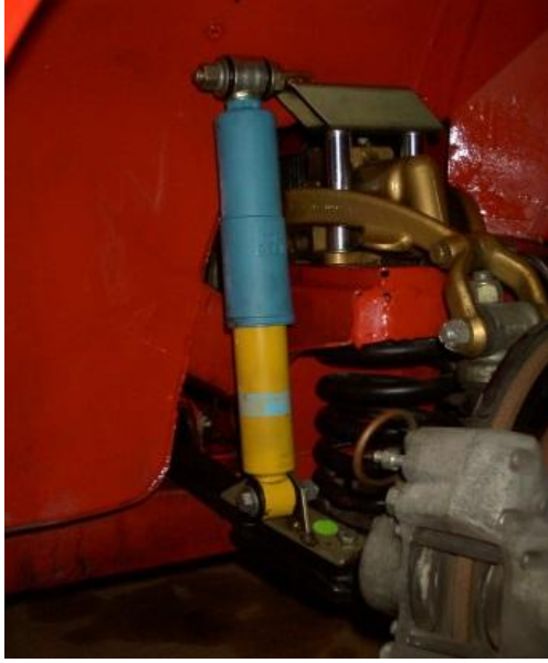
Front Right Installation. Shock is installed BEHIND the spring.
