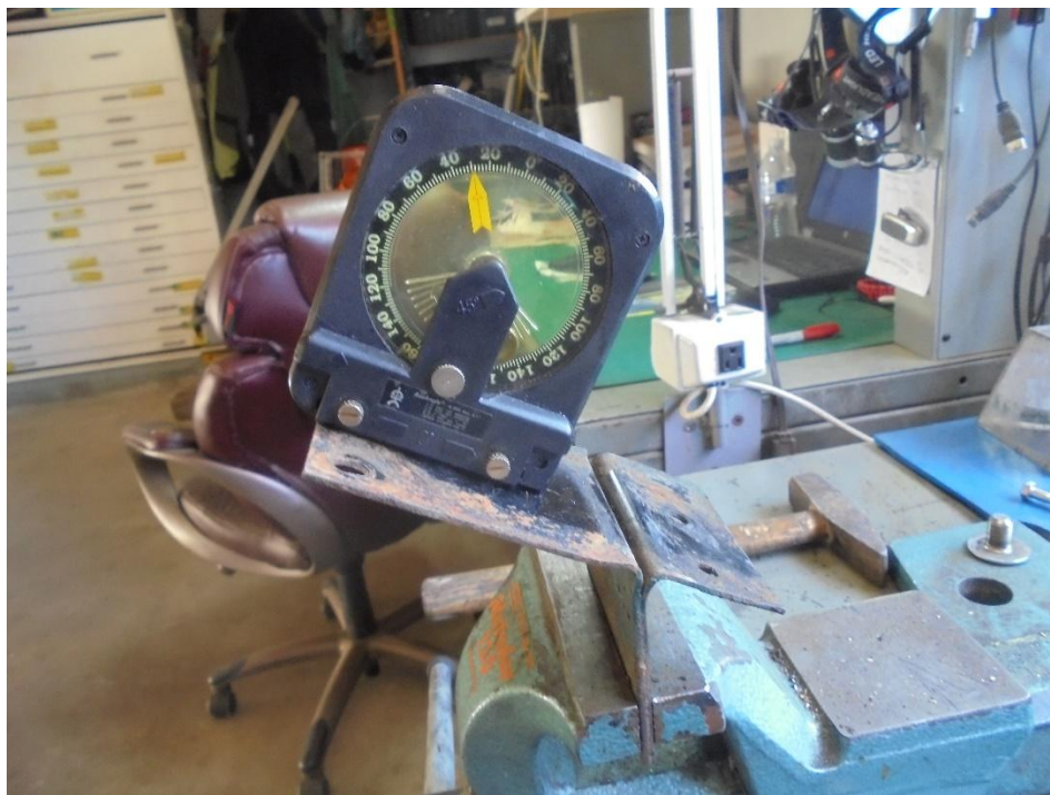
MODIFICATION OF ORIGINAL BRACKET, BEND TO 30 DEGREES
