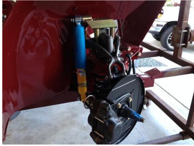
Front Right Installation. Shock is installed BEHIND the spring.
